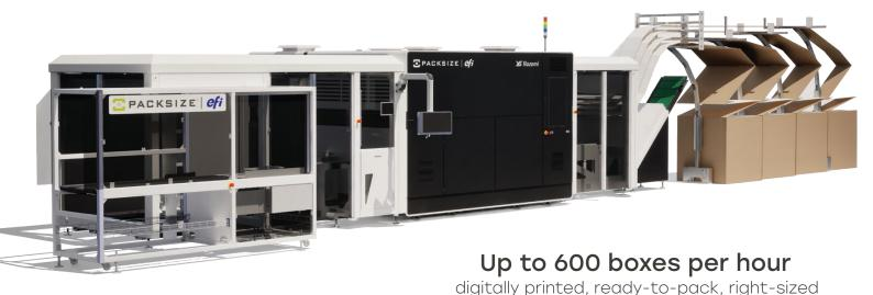
The efficient, fully automated Packsize® EFI™ X5® Nozomi system produces full colour, ready-to-pack, right-sized boxes on-demand. The first of its kind, the X5 Nozomi streamlines and enhances sustainable packaging production environments, while providing a more exciting and attractive unboxing experience for the end-user.
